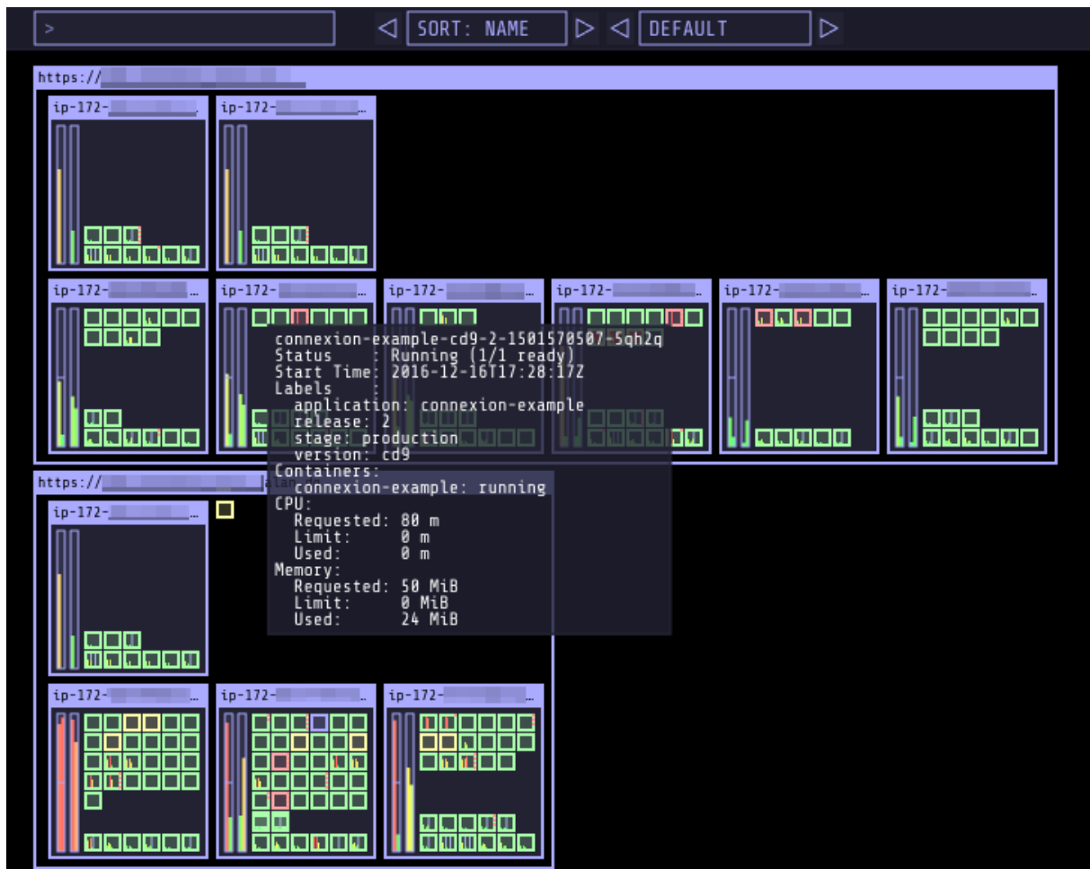
Figure 1: kube-ops-view is a read-only system dashboard which gives you a bird's-eye view for multiple Kubernetes clusters
